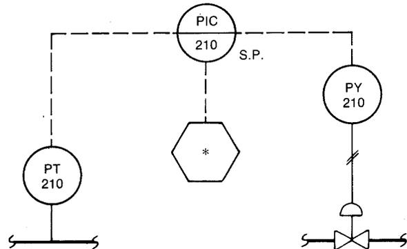
Figure A12. Supervisory Set Point Control—Analog Controller Complete with Conventional Faceplate. Computer Supervisory Set Point Hardwired.
