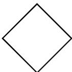
**4.4.2** Distributed control interconnecting logic controller with binary or sequential logic functions.
