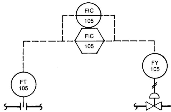
Figure A2. Computer Control—With Analog Backup
