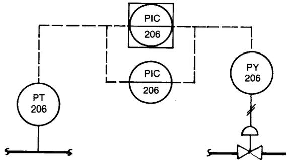
Figure A8. Shared Display/Shared Control—With Analc Controller Backup
