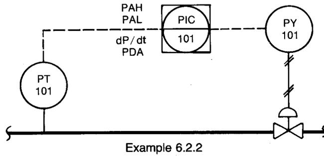
**6.2.3** Alarms on controller output shall use the undefined variable identifier X, i.e.:
